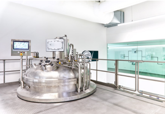
The centerpiece is the mixing plant. 30,000 litres of aloe vera gel are produced per day and stored in our 6.50-meter-high containers.
