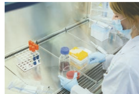
Employee Stefanie Jaszka conducts the examination for the determination of the intestinal bacterium Escherichia coli .
